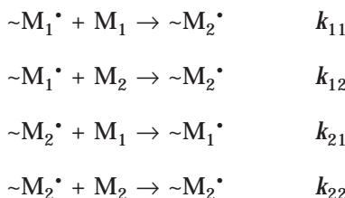
with  $r_{12} = k_{11}/k_{12}$ ,  $r_{21} = k_{22}/k_{21}$ , where  $\sim M \cdot$  represents a polymer chain ending with a radical derived from monomer M.
